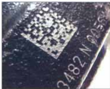
Surface irregularities (pits) on cast surfaces can make marks difficult to read. The pits create shadows that can be misinterpreted by the imager as dark elements of the symbol.
