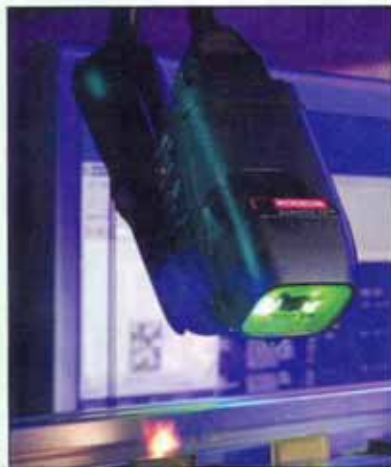
Stationary imagers can be permanently installed at the appropriate focal distance and angle for optimal lighting to read low contrast direct part marks.
