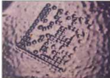
Dot peen marks rely on changes in depth to create the light and dark elements of a Data Matrix symbol.
