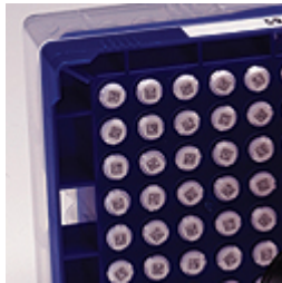
Figure 10. Miniature megapixel imagers can read up to 100 data-matrix symbols within a single image capture.
