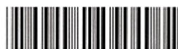
Figure 2. A linear bar code is a series of parallel bars and spaces.
