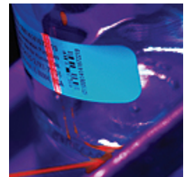
Figure 9. In order for a linear imager to read a bar code, the laser's field of view must be aligned perpendicularly to the code's bars and spaces.
