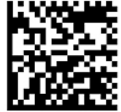
Figure 3. A data matrix is a 2-D code made of light and dark circular or square elements.
