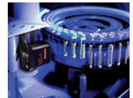
Figure 1. Embedded bar code readers automate the data-entry process for instruments such as clinical analyzers.
